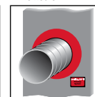
5. Leave completed seal undisturbed for 48 hours.
