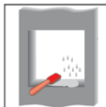
1. Clean penetration. Pre-moisten sides of penetration.
