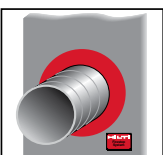
5. Fasten identification plate (if required)
